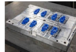
With multi-cavity tools, even high quantity runs are possible if there is concern for sudden spikes in demand
