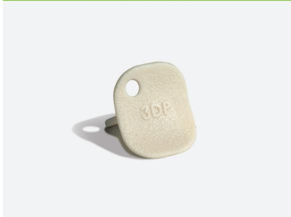
In 3DP an inkjet print head moves across a bed of powder, selectively depositing a liquid binding material, and the process is repeated until the complete part has been formed. After completion, the unbound powder is removed leaving the finished object.
