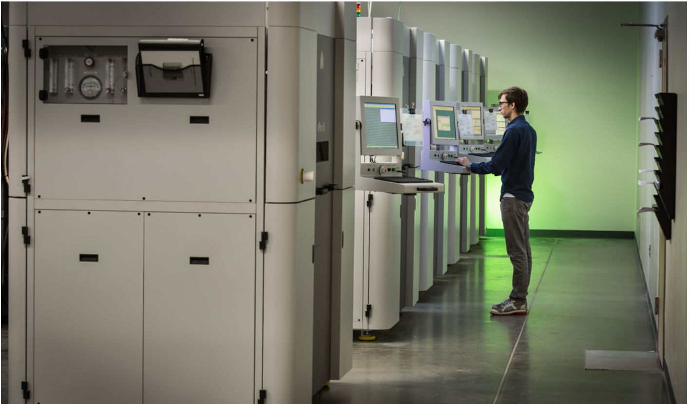
3D Systems units print plastic SLS parts at Protolabs' facility in Raleigh, North Carolina.
