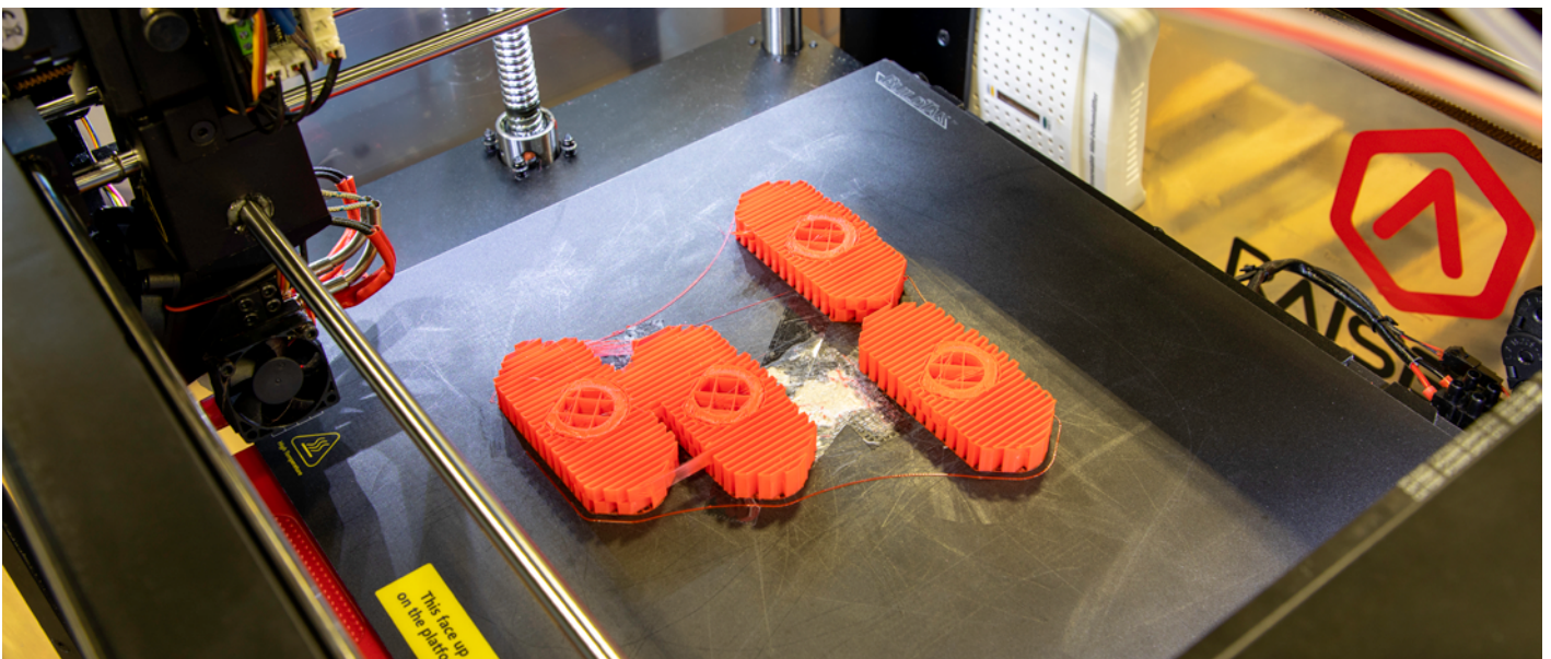
Parts produced using fused deposition modeling (FDM). FDM machines offer a greater number of material options than other 3D printing processes.
