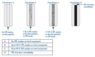
The second character describes if the TPE strip will tear during the measurement at any position on the peel path.
