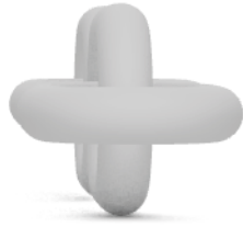
Figure 8: Chain links oriented at 0 and 90 degrees to the print bed
