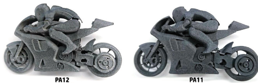
Figure 1. Look and feel of two identical parts printed with HP PA 12-Balanced (left) and HP PA 11-Mechanical (right)
