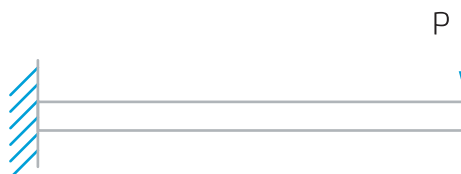
Figure 10. Cantilever beam with a point-applied end load
