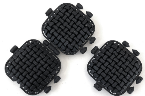
Figure 3: Another type of hinge uses cones that fit into matching divets. These modules by can snap apart and back together.
