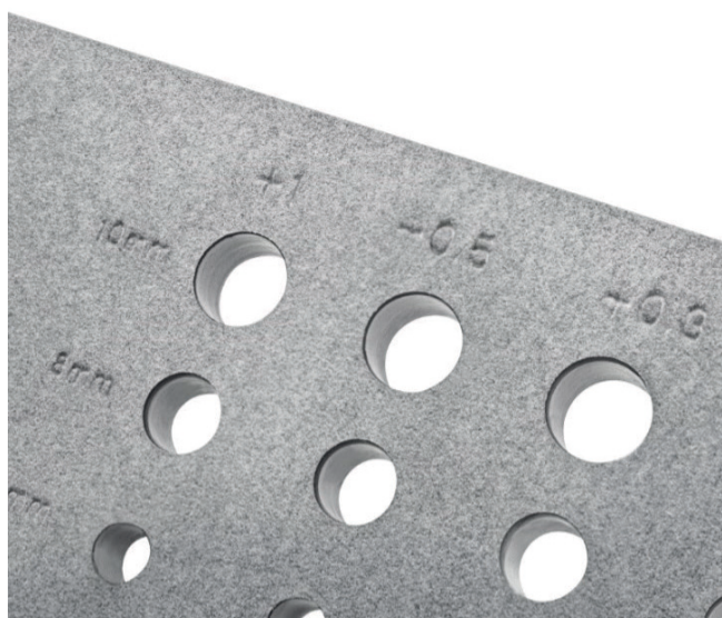
Figure 2: HP MJF pre-formed hole testing
